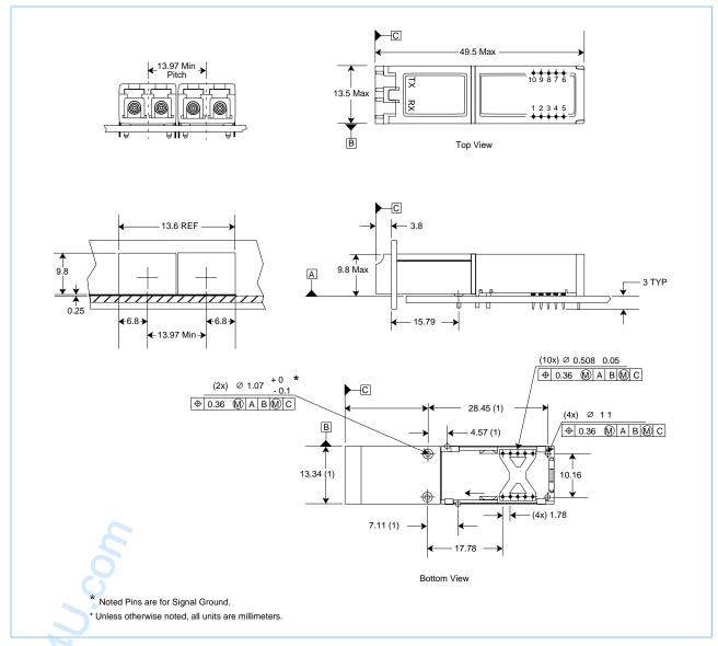
The SFF-1063/1250N-SW is intended to be used on a host card having a thickness of 0.062" to 0.100". The host card footprint with essential keepouts and drill holes is shown in Host Card Footprint on page 14.
